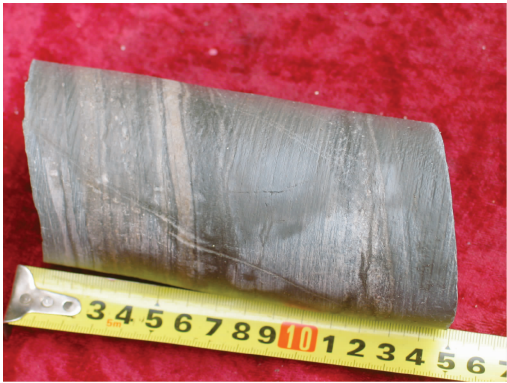
图 1 通南巴地区白色硬石膏岩与灰色白云岩互层沉积(川涪 82 井, T_1f^2 ) Fig. 1 Interbedded white anhydrite and grey dolomite in Tongnanba area( T_1f^2 , Well CF82)
