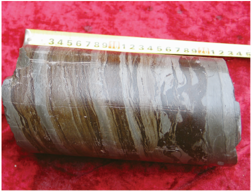
图 2 通南巴地区棕红色膏盐岩夹灰色粉晶云岩条带(川涪 82 井, T_1f^5 ) Fig. 2 Brownish red evaporate with grey dolomite interbed in Tongnanba area( T_1f^5 , Well CF82)
